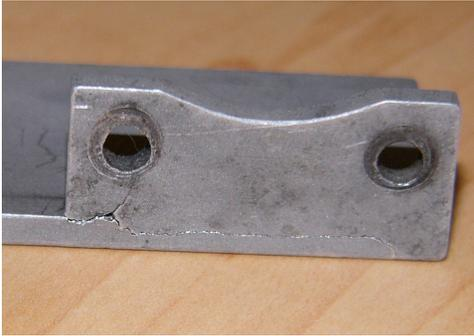
**Figure 24 - Crack propagation in the snake arm**
