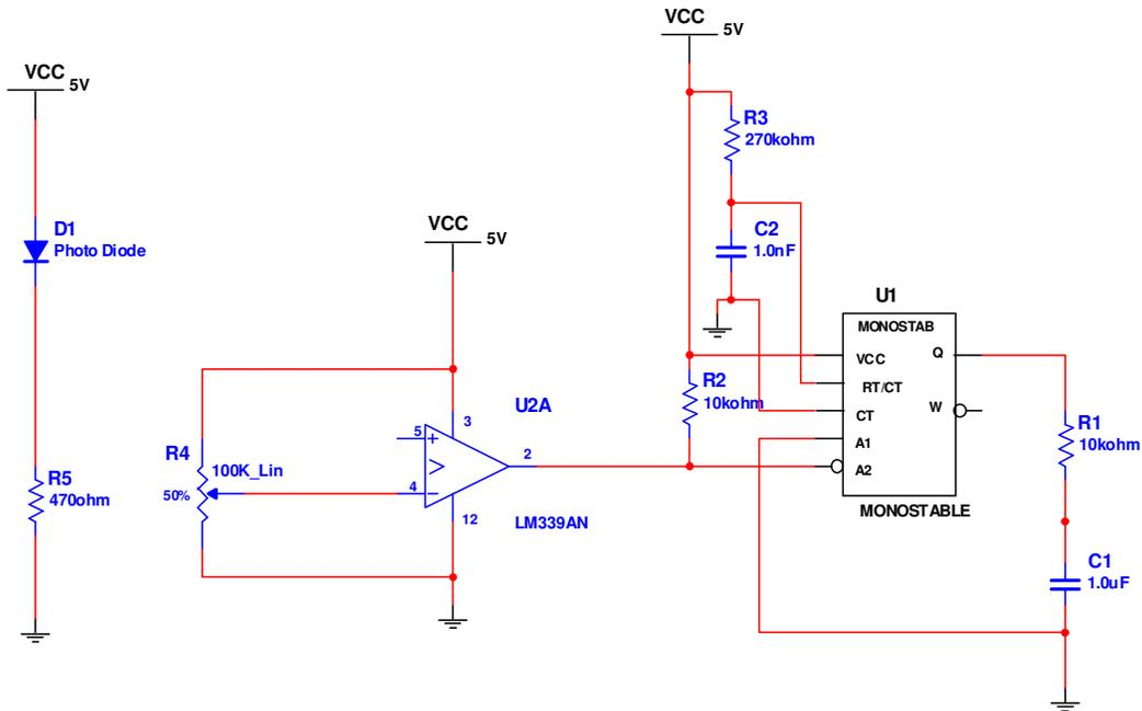
Figure 21 - Frequency to voltage converter circuit diagram
