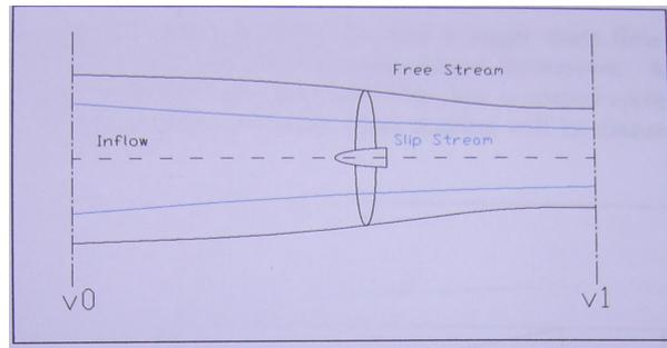
Figure 1 - Flow around a rotor with out duct
