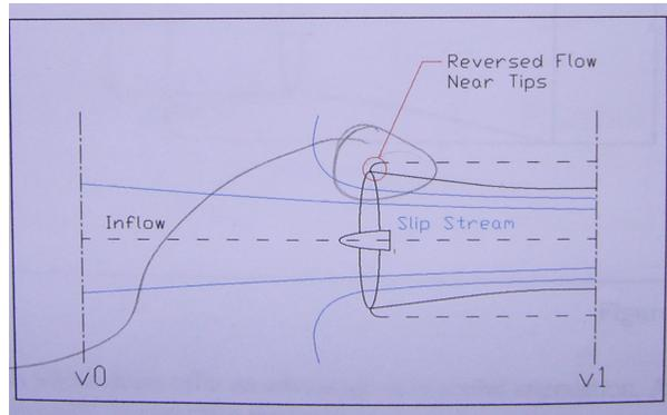
Figure 2 - airflow around an open Lower stream duct
