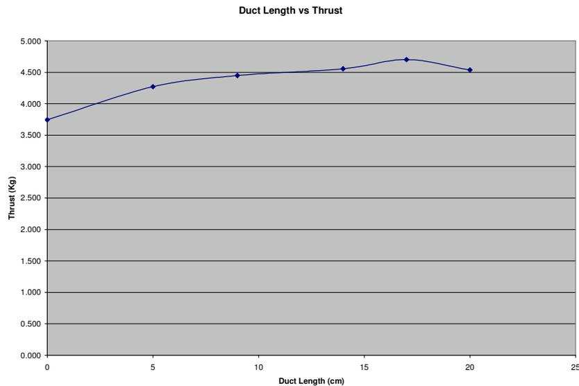
Figure 8 - Graph of Duct Length vs Thrust
