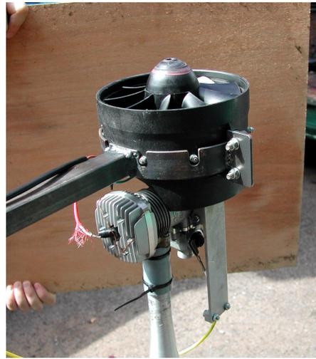
Figure 14.5.6: Thrust IC with Ducted Fan
