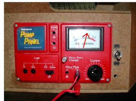
13. Turn Pot 3 until the GENSET turns repeatedly and hold. Once the engine fires to 0%.
