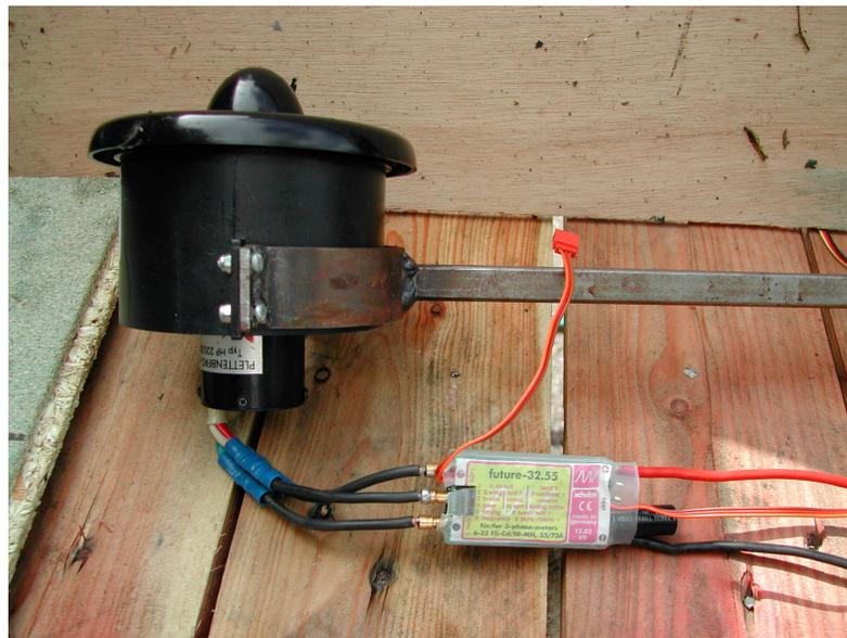
Figure 5.2: Plettenberg HP220/30/A4 S P4, and Schulze Future 32.55 controller
