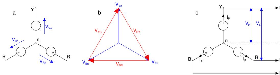
Figure 6.16: Star Phasors and wiring
