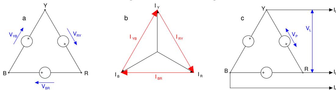
Figure 6.17: Delta Phasors and wiring
