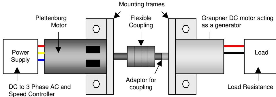
Figure 6.12: Rig for Graupner Motor testing
