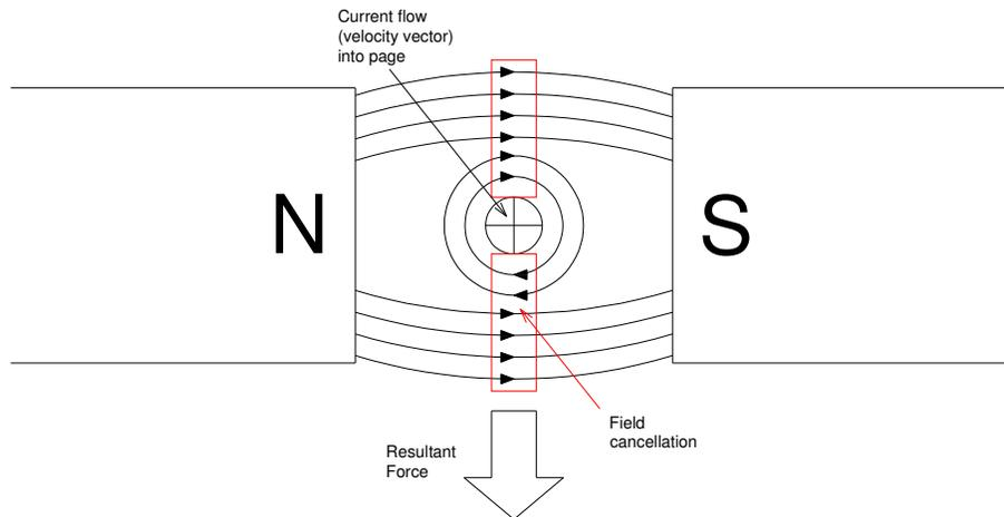
Figure 6.4: Effect of a current carrying conductor in a magnetic field.
