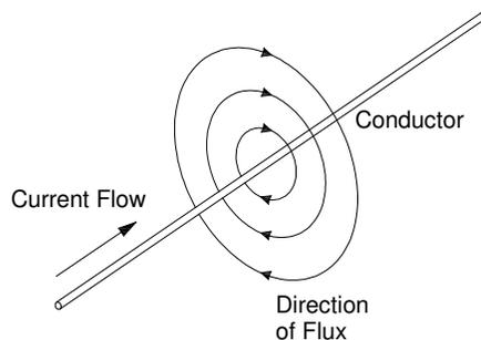
Figure 6.3: Flux lines around a current carrying conductor
