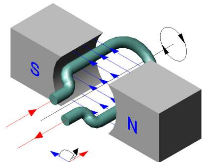
Figure 6.6: DC motor, stage 2
