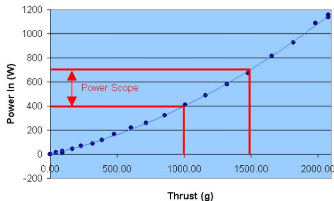
Figure 6.1: Electric Perimeter Fans, thrust vs. power consumed
