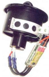
*Figure 2.1: Propulsion Ducted Fan using a WeMoTec Midi Fan powered by a Plettenberg HP 220 motor [6]*
