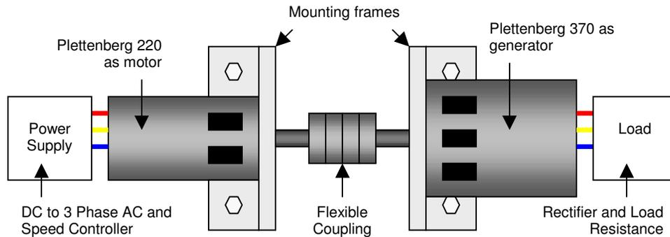
Figure 6.13: Rig Plettenberg HP 370 Motor testing
