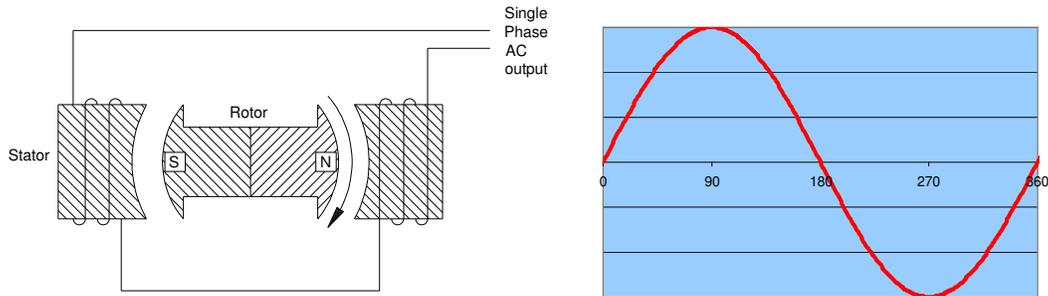
Figure 6.14: Output from a basic single phase generator
