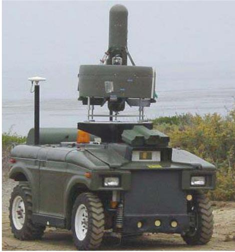
**Figure 3<sup>6</sup> : UAV on Carrier/Launcher**
